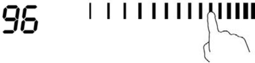
6. When the cooking time expires, the buzzer will beep for 30 seconds and the timer indicator will show "00".
