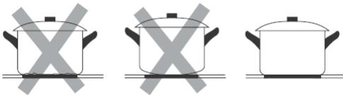
Make sure that the base of your pan is smooth, sits flat against the glass, and is the same size as the cooking zone. Use pans whose diameter is as large as the graphic of the zone selected. Using a pot a slightly wider energy will be used at its maximum efficiency. If you use smaller pot efficiency could be less than expected.
