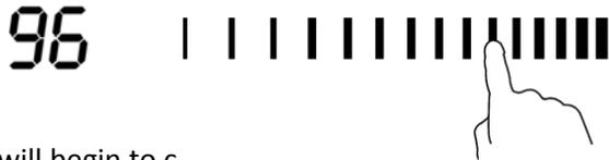
6. When the time is set, it will begin to c immediately. The display will show the remaining time and the timer indicator flash for 5 seconds.
