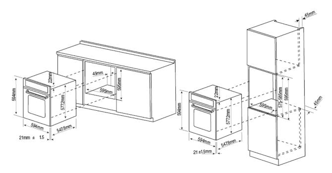
NOTE: Dimensions provided above for the cut-out are for a face mount only!
