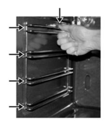
To remove the side support racks, push down on the wire below the locking pin and pull away from the oven wall until you can release the bottom of the support from the holes in the oven wall. To replace, reverse this procedure.
