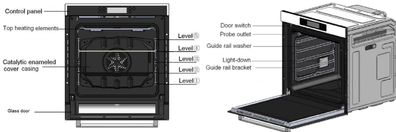
Shelf levels are numbered from the bottom up. Levels 4 and 5 are used mainly for the grill function. Please refer to the suggested levels, functions and temperatures.
