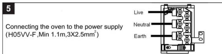
The earth wire must be connected to the
