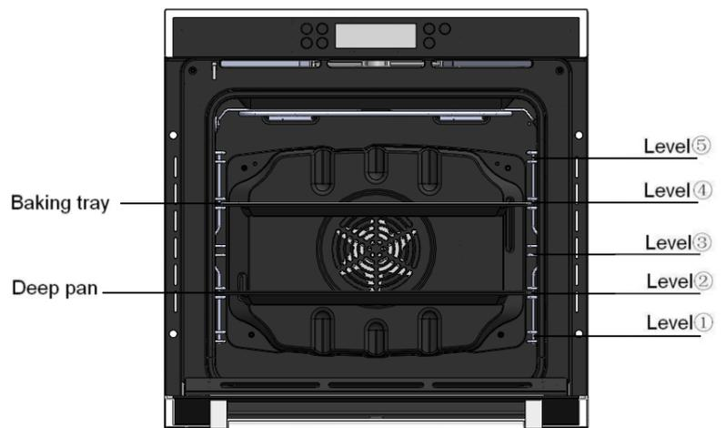
When using the deep pan or the baking tray to collect drippings from cooking foods, ensure that the pan or tray is properly placed in the side runners. Allowing these accessories to come in contact with the bottom surface of the oven can damage the enamel of the surface. Trays and pans placed on level 1 should clear the bottom surface of the oven by at least 2 cm.
