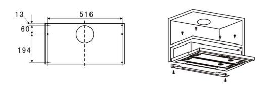
**Step 1:** The rangehood should be placed at a minimum distance of 65cm above the cooking surface when placed above an electric hob and a minimum of 75cm above the cooking surface when placed above a gas cooktop.
