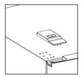
3. Take off the upper door, take out the screw from the middle hinge by cross screwdriver, then take off the lower door.
