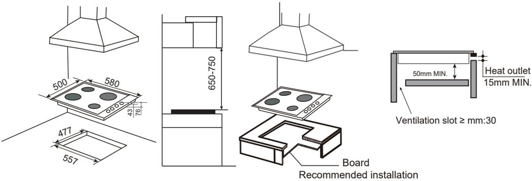
**Note:** no overhead ventilation system is to be installed within 650mm from the top of the hob.
