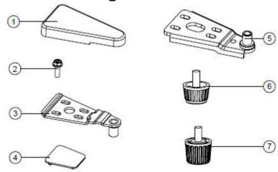
1)Door hinge cover 2)Flange screw 3)Door hinge 4)Cap 5)Lower door hinge 6)Short cabinet foot 7)Height cabinet foot
