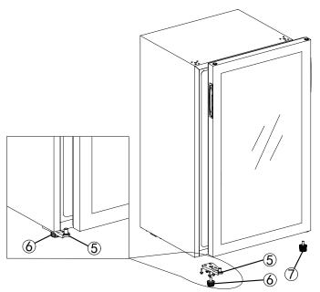
5) Fit the lower door hinge 5 to the down left corner; Install the short cabinet foot 6 and the height cabinet foot 7. Put the door above and insert into the lower door hinge.
