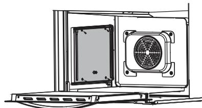
Removing the catalytic liners
