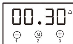
3. 5 seconds after the time is set, the signal function "Δ" is on. Your setting is saved. Or alternatively set the time and press button 2 immediately after to set the timer.
