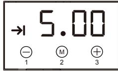
2. Cooking time automatically changes to 3:00.5 seconds after the setting, the auto function is on. 3 hours later, the current time shows "5:00" the alarm signal is activated.
