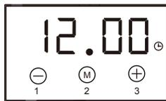
2. The current time can be set with button 1 and 3, 5 seconds after the time has been set, the new data will be saved.
