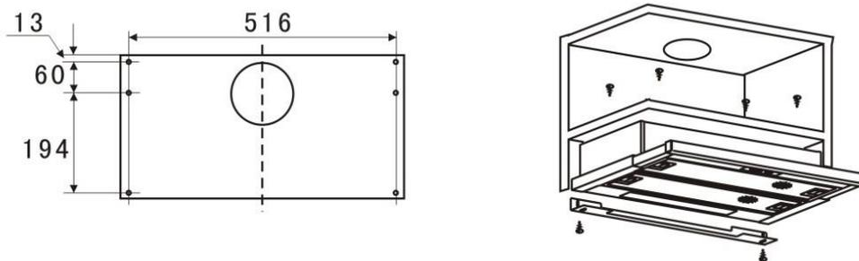
**Step 1:** The rangehood should be placed at a minimum distance of 65cm above the cooking surface when placed above an electric hob and a minimum of 75cm above the cooking surface when placed above a gas cooktop.
