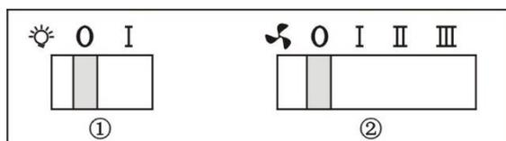
1. ① represents the light. Push the switch to “I” to turn the light on, and “0” to turn the light off.
