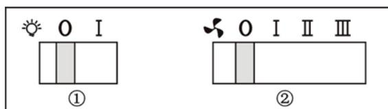
1. ① represents the light. Push the switch to “I” to turn the light on, and “0” to turn the light off.
