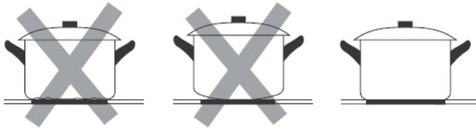
Make sure that the base of your pan is smooth, sits flat against the glass, and is the same size as the cooking zone. Use pans with a base diameter that is as large as the graphic of the zone selected. By using a slightly wider pot, energy will be used at its maximum efficiency. If you use a smaller pot, the efficiency could be less than expected. Pots less than 140 mm could be undetected by the hob. Always centre your pan on the cooking zone.
