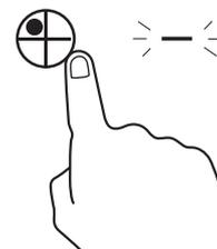
2. Turn the cooking zone off by scrolling down to “0” using the “-” regulating control.
