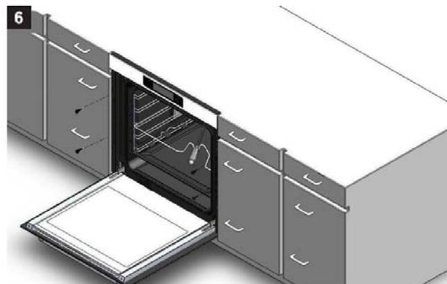
Do not use the door as a handle when lifting the unit into place as this may damage the hinge assembly. Use the lifting handholds placed on either side of the oven
