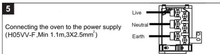
The earth wire must be connected to the (⏏) terminal of the oven.
