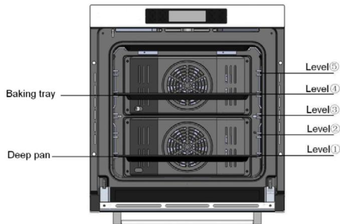
When using the deep pan or the baking tray to collect drippings from cooking foods, ensure that the pan or tray is properly placed in the side runners. Allowing these accessories to come in contact with the bottom surface of the oven can damage the enamel of the surface. Trays and pans placed on level 1 should clear the bottom surface of the oven by at least 2 cm.
